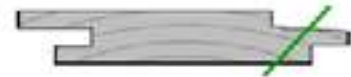
Secret nail shiplap boards in cross section showing proposed fixing position of the screws
